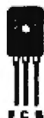
BD131 NPN BD132 NPN BD135 NPN BD136 PNP BD137 NPN BD138 PNP BD139 NPN BD140 PNP
