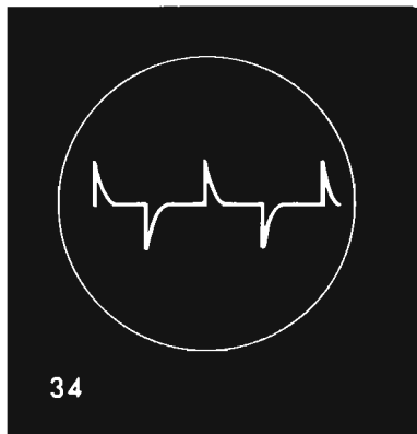
Trace 33) Effect of long time constant on a square wave; Trace 34) Effect of short time constant on a square wave.
