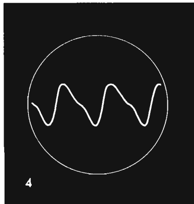
Trace 3) 15% 2nd harmonic -90^\circ out of phase; Trace 4) 30% 2nd harmonic in phase.
