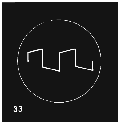
Trace 33) Effect of long time constant on a square wave; Trace 34) Effect of short time constant on a square wave.
