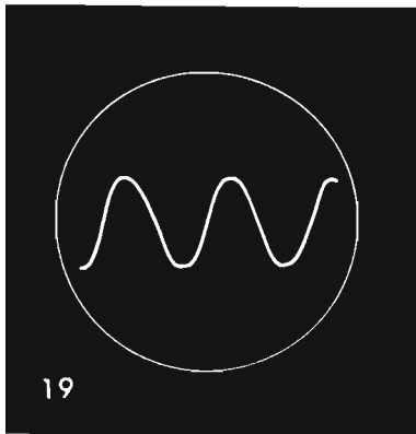
Trace 19) 5% 2nd harmonic in phase and 5% 3rd harmonic in phase; Trace 20) 5% 2nd harmonic in phase and 15% 3rd harmonic in phase.
