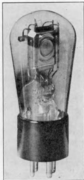
FIG. 39. A three-electrode high-vacuum tube designed to have a minimum of undesired disturbances in the plate current flow; that is, a "low-noise" tube.
