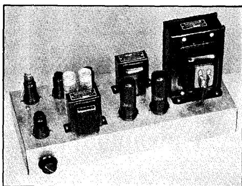
FIG. 1204 — METAL-TUBE SPEECH UNIT WITH PUSH-PULL 6L6 OUTPUT
