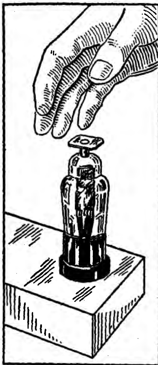
FIG. 37.—If a sensitive current indicator be connected as shown in fig. 36, the meter will show the current change due to the capacity effect, if a hand be placed in proximity to the antenna.
