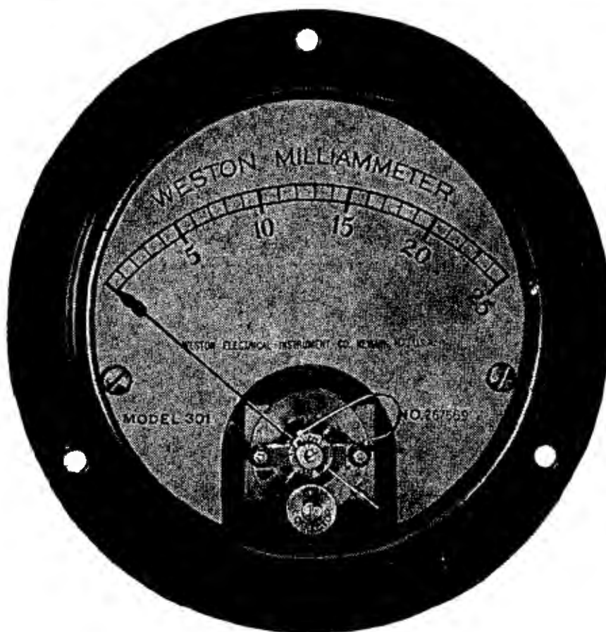
FIG. 3.—Weston plate or grid milli-ammeter for measuring the plate current of vacuum tubes. It will give a deflection for steady or pulsating direct current and will indicate the average value of a pulsating current. Superimposed upon the steady plate current is the current due to the modulation which is an alternating current and will cause the total plate current to be a pulsating current varying at the same frequency as the modulation current. The milli-ammeter will again indicate the average value of this current and if the tube be working at a point where it rectifies, this average value will not be the same as the value of the unmodulated steady plate current and therefore fluctuate with the modulation. For perfect reproduction, amplifying tubes should not rectify and no variation in the indication of the milli-ammeter should occur. In practice however, on account of the properties of vacuum tubes, some rectification will result, but by properly adjusting the grid bias, a minimum fluctuation in the plate current may be obtained consistent with good quality and volume.
