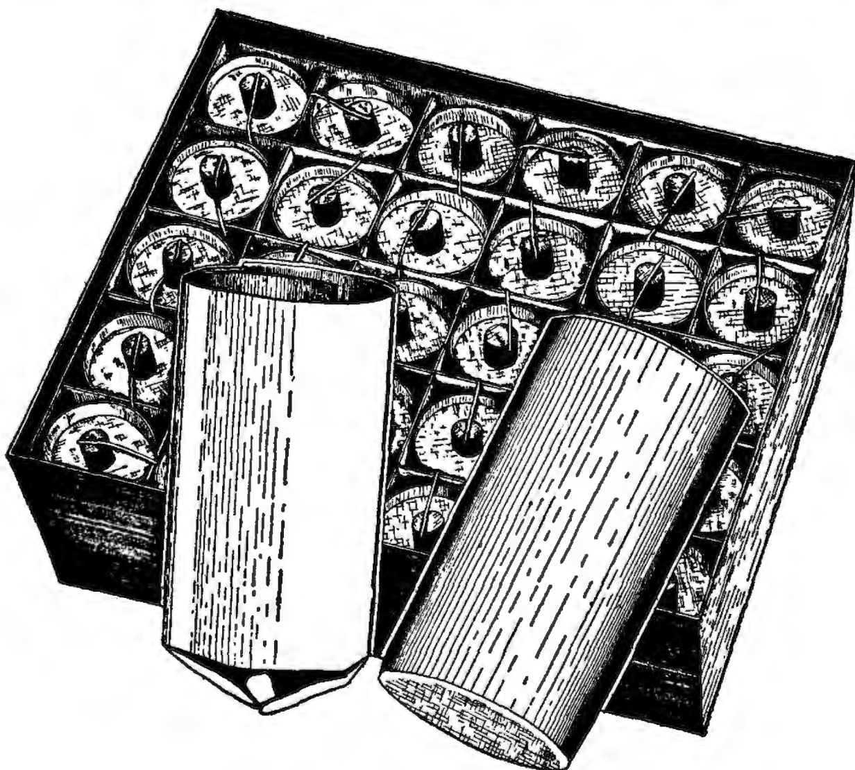
FIG. 5.—Kleartone dry battery with top removed showing what the inside of a 45 volt B battery looks like. The illustration also shows at the right the one piece seamless zinc cup, and at the left the paper insulator and filter which fits inside it.
