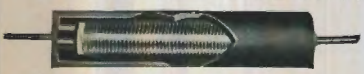
Cross Section — showing progressive inter-leaved windings for higher resistance values in less space.
