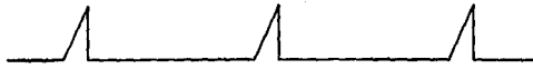
FIG. 15-51.—Wave form of sweep voltage used when it is desired to observe only a portion of the cycle of voltage impressed upon the oscilloscope.
