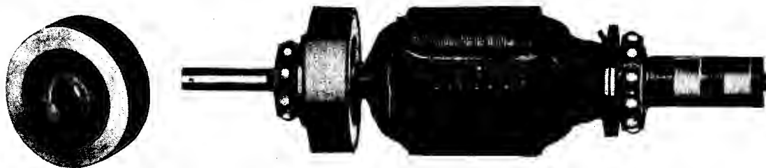
Wound rotor, with damper for Selsyn Model 2JD55JA1. Left: View of damper removed
