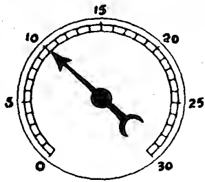
3. Loose valve guides. See also Nos. 2 and 4.
