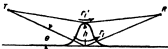
FIG. 22-9. Ground-reflected rays with and without an obstacle at the reflecting point. For the sake of clarity the heights of the obstacle and the antennas are greatly exaggerated.
