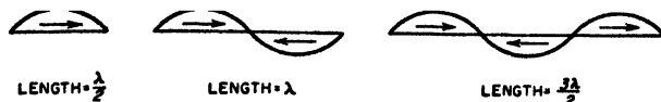
FIG. 23-3. Typical current distributions in resonant lines. The distributions shown have been idealized by assuming zero losses.
