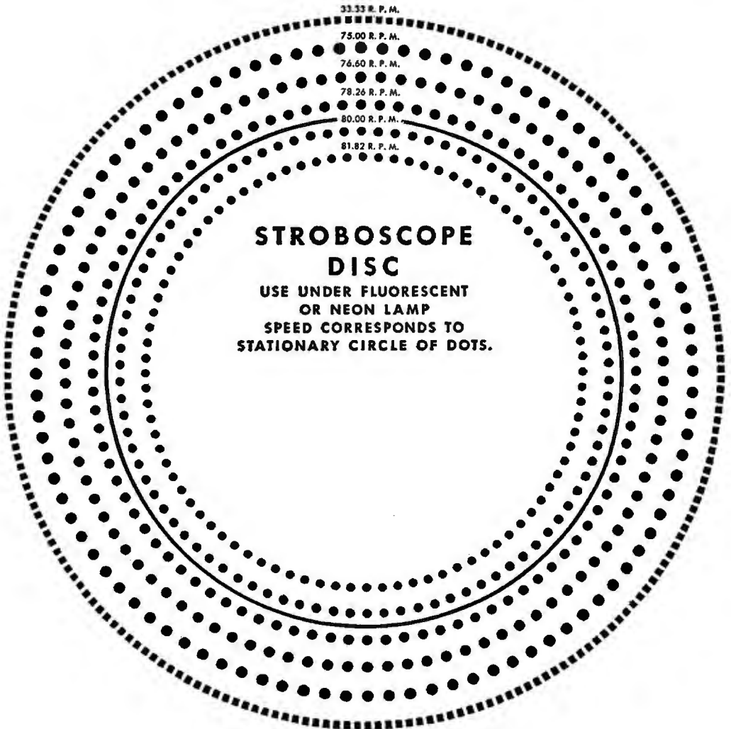
Fig. 12-18.—Stroboscope disk used in regulating speed of phonograph motors.
