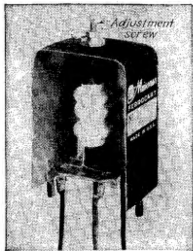
FIG. 14-13.—Universal adjustable replacement RF or antenna coil.
