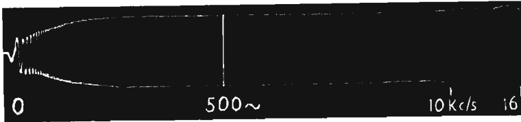
FIG. 17/2.—Oscillogram of response of amplifier, exposing distortion at 10–15 Kc/s.
