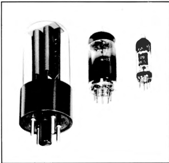
Subminiature Tube Compared with Standard Tube
