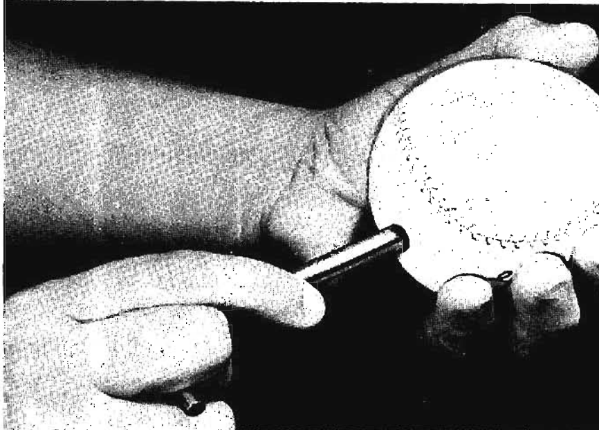
Fig. 85—To drill hole for the shaft in the rubber ball use a solid ball and "cork borer."
