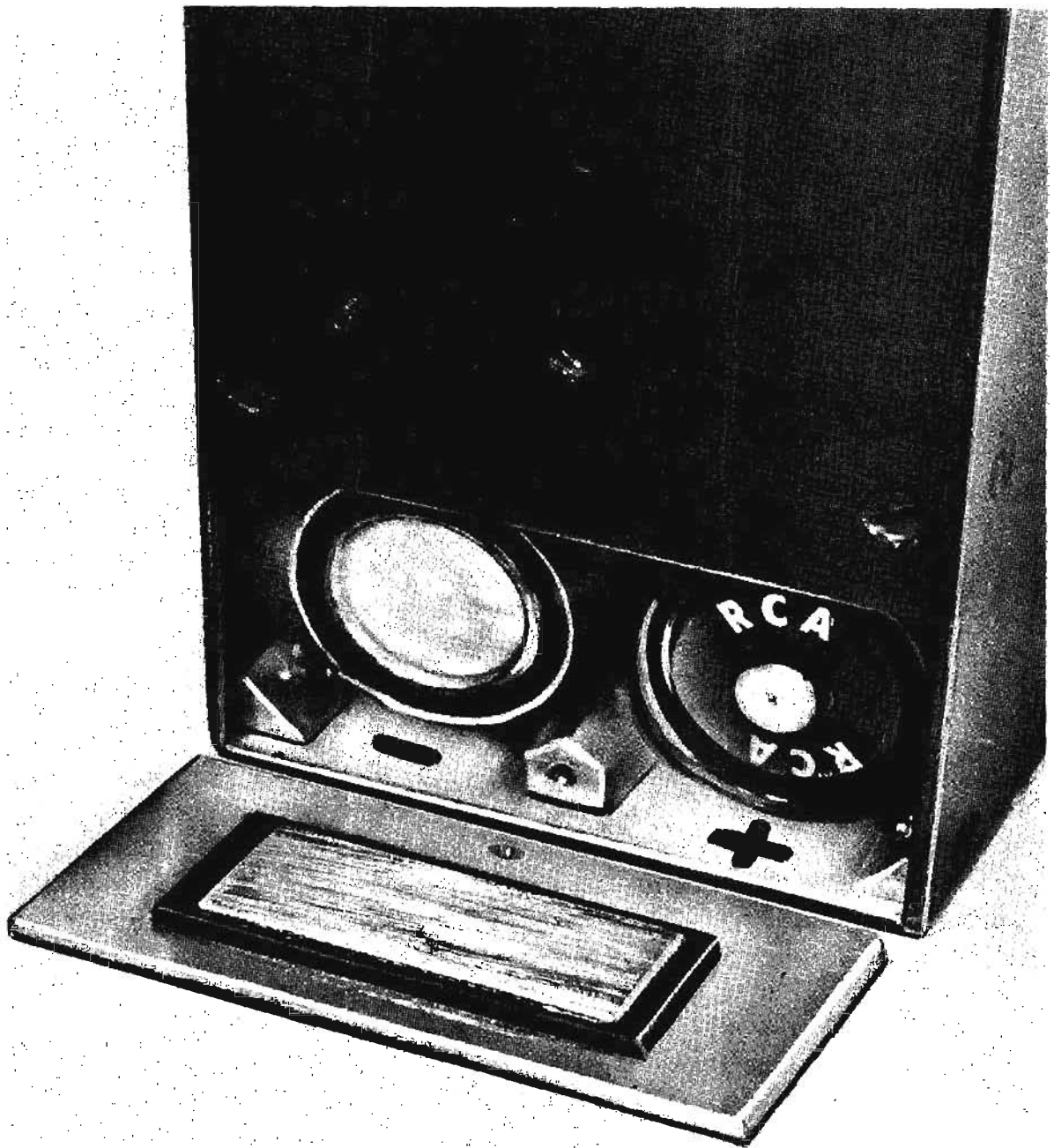
Fig. 166—Battery compartment with batteries installed.
