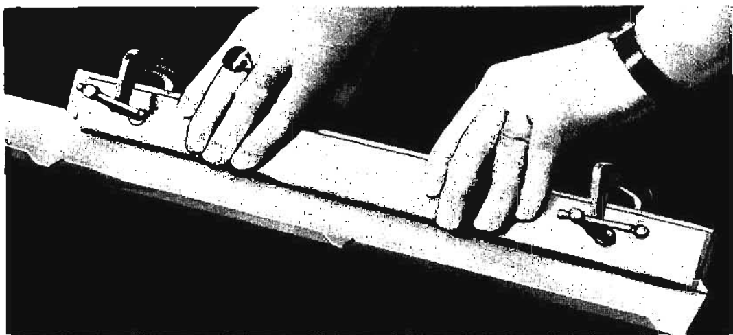
Fig. 46A—Bending sides of aluminum for chassis.
