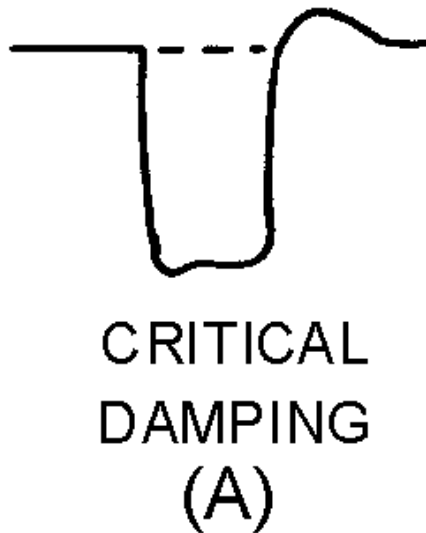
Figure 3-36A.—Waveform damping. CRITICAL DAMPING.
