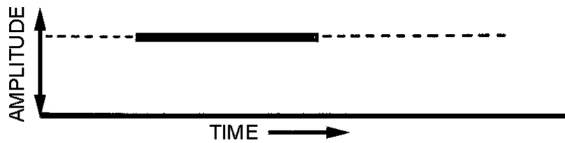
(B) RESPONSE OF AM DEMODULATOR TO SIGNAL
