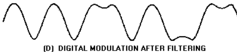
Figure 2-26D.—Simulated phase-shift keying. DIGITAL MODULATION AFTER FILTERING.
