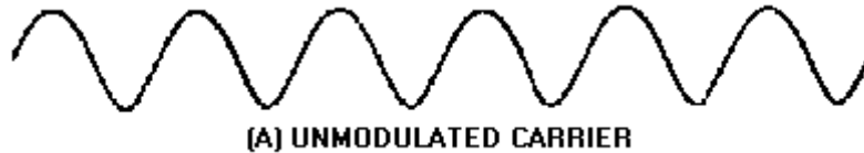
Figure 2-25A.—Phase-shift keying. UNMODULATED CARRIER.
