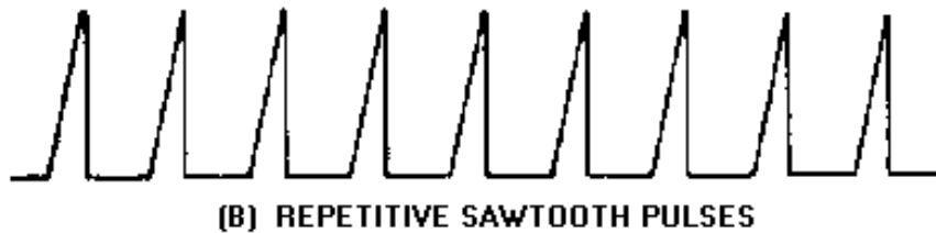
Figure 2-44B.—Pulse-duration modulation (pdm). REPETITIVE SAWTOOTH PULSES.
