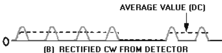
Figure 3-1B.—Cw demodulation. RECTIFIED CW FROM DETECTOR.
