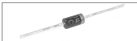
1N4004 diode. Band identifies cathode, or (+) end.
